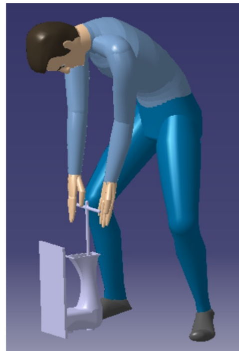
Fig. 3. Posture opted by the worker for vertical hole tapping in sewing machine body cast.
